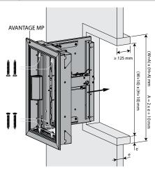
1. Put glue type CF GLUE on the uprights and cross pieces and between the lining and the wall. Screw the sleeve using chipboard screws Ø5 x 70 mm at 150 mm intervals.
