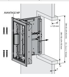
1. Put glue type GLASROC F V500 on the uprights and cross pieces and between the lining and the wall. Screw the sleeve using chipboard screws Ø5 x 70 mm at 150 mm intervals.
