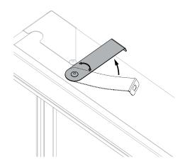
1. Rotate the four fastening plates on the damper 90° (to the upright position).
