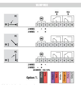
**DC:** Switch closed position smoke evacuation shutter
