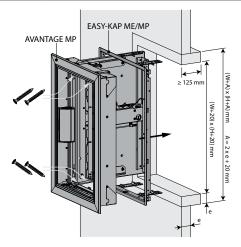
1. Coat the edges of the opening with adhesive plaster. Seal the joints between uprights and cross pieces and between the lining and the wall with vegetable fibre caulking and plaster.
