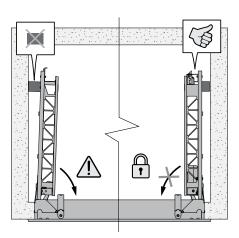
2. Be sure to cut the block to the correct dimensions so that the blocking mechanism can engage when the door opens.
