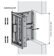
2. Make an opening with dimensions (W+10) x (H+10) mm. Fix the shutter in the opening using 4 screws and dowels  $\emptyset$ 6 x 40 mm.
