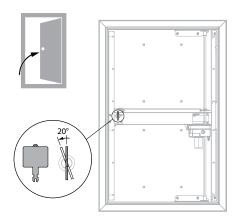
1. Unlocking 1V Turn the key 20° anti-clockwise and push the shutter into its open position.
