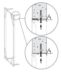
2. The mounting frame should always be fastened to the concrete shaft with screws and dowels (Ø6 x minimum 60 mm, steel or stainless steel).
