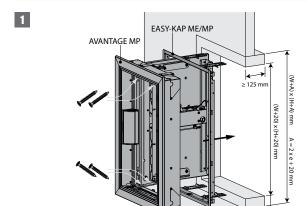
1. Make an opening with dimensions (W+A) x (H+A) mm. A = 2 x thickness sleeve (e) + 20 mm min. / + 30 mm max. Fit a sleeve of the same type of material and thickness as the duct (thickness e) of minimum 125 mm deep in the opening. Fasten and seal the mounting frame. See details per type of shaft hereafter.
