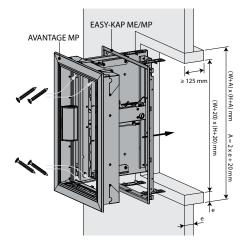
1. Coat the edges of the opening with adhesive plaster, type FACILIS.
