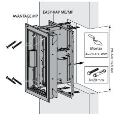
1. In case the mounting frame is screwed: Make an opening with dimensions (W+20 min / +30 max) x (H+20 min / +30 max) mm.
