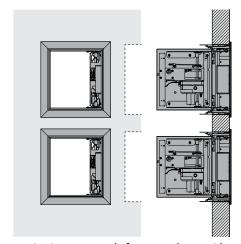
3. When mounting in a concrete shaft, you need to provide a continuous reinforcement in the vertical columns of at least  $4 \times \emptyset 8$  mm.
