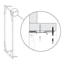
2. Two fixing lugs are provided at the bottom and at the top of the mounting frame: fold these against the sleeve. When fixed with screws, fasten the mounting frame to the sleeve with chipboard screws ( $\emptyset$  6 x e) mm. These screws can be fixed in one of the openings provided for this purpose, depending on the depth of the sleeve. Take care not to misshape the frame during its installation. The finished opening must have the same size as the mounting frame (W+10) x (H+10) mm.
