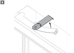
4. Rotate the four fastening plates on the damper  $90^{\circ}$  (to the upright position).
