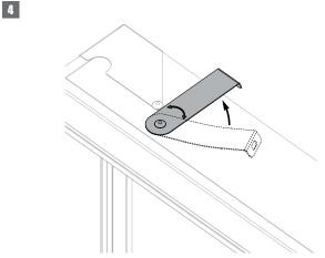
4. Rotate the four fastening plates on the damper 90° (to the upright position).
