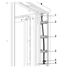
4. Lead the cables through the opening. Use the protective sleeve (1), the fixation clips (2) and the plastic cable clamp (3) to attach the cables to the frame. Lead the cables to the connection box through the grommet (4) and connect according to the electrical connection diagram.
