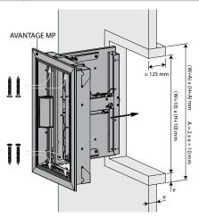
1. Assemble the sleeve with staples and affix the assembled sleeve to the shaft wall with staples.
