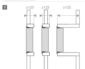
1. The shutter is affixed to the smoke control shaft through a sleeve. That sleeve can be installed either in the shaft, in the axis of the shaft or outside the shaft (or shaft extension).
