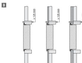
3. In order to prevent cracks around the opening in the long term, a finishing layer (plasterboard, (cellular) concrete, rigid wall) can be added between the mounting frame and the opening.
