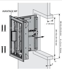
1. Coat the edges of the opening with adhesive plaster, type FACILIS
