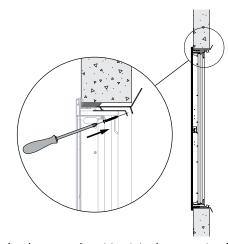
5. Open the shutter and position it in the mounting frame. Fasten the shutter onto the mounting frame with the 4 screws supplied, as shown in the drawing. Tightening the screws pulls the shutter towards the wall until its final position. You can also slightly correct the angle of the shutter with respect to the mounting frame.
