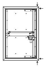
1. The electrical connection is possible via the 2 corners at the side of the hinges.
