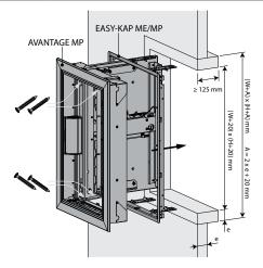
1. Put glue type CF GLUE on the uprights and cross pieces and between the lining and the wall. Screw the sleeve using chipboard screws  $\emptyset$ 5 x 70 mm at 150 mm intervals. Two fixing lugs are provided at the bottom and at the top of the mounting frame: fold these against the sleeve. First coat the opening with glue CF GLUE. Glue the mounting frame to the lining taking care not to misshape it. The finished opening must have the same size as the mounting frame (W+10) x (H+10) mm.
