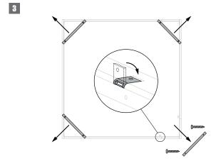
3. Put aside the screws that are affixed to one of the cross slats, then unscrew the 4 cross slats of the mounting frame and fold the 8 fastening plates in the frame.
