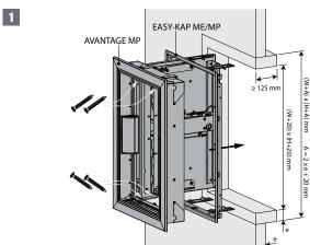
1. Coat the edges of the opening with adhesive plaster type PLACOL (in case of Geoflam) or GEOCOL (S) (in case of Geotec). In case of Geotec you can also assemble the sleeve with glue and screws Ø 5 x (2 x e) mm and affix the assembled sleeve to the shaft wall with glue and screws Ø 5 x (2 x e) mm every 100 mm. Seal the joints between uprights and cross pieces and between the lining and the wall with vegetable fibre caulking and plaster or with GEOCOL (S) (in case of Geotec).
