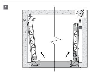
1. Shock absorber (foam) comes standard with the shutter. It can be affixed to the inner face of the door to prevent it from hitting the shaft wall when opening.
