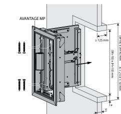
1. Coat the edges of the opening with adhesive plaster type PLACOL (in case of Geoflam) or GEOCOL (S) (in case of Geotec). Seal the joints between uprights and cross pieces and between the lining and the wall with vegetable fibre caulking and plaster or with GEOCOL (S) (in case of Geotec).
