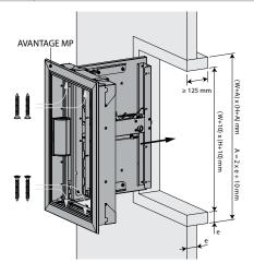
1. Coat the edges of the opening with adhesive plaster. Seal the joints between uprights and cross pieces and between the lining and the wall with vegetable fibre caulking and plaster.
