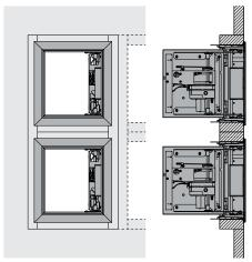
1. The shutters can be installed at minimal distance on top of or next to each other, if they are mounted in separate sleeves made from the shaft material with the required fire resistance. It is advised not to exceed a 4 x 2 configuration (W x H).
