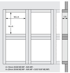
2. In case several shutters are mounted at a minimal distance, the bearing and reinforcement points of the shaft must be adjusted in proportion to the increased weight. The installation of the shaft must comply with the classification report delivered by the shaft manufacturer.
