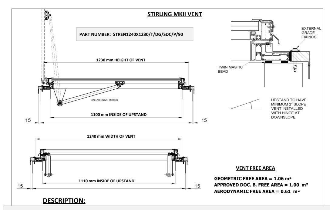
STIRLING MKII CASEMENT VENT," ROOF APPLICATION (W)1240mm X (H) 1230mm TURN DOWN BASE 28mm STD DOUBLE GLAZED, TOUGHENED OUTER, LAMINATED INNER, SPINDLE ACTUATOR OPERATION 24V DC OPEN/CLOSE 90 DEGREE OPENING - PAINTED TO (RAL)
